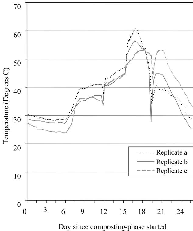
Fig. 1. Temperature profiles of the CV-system during the composting-phase.
