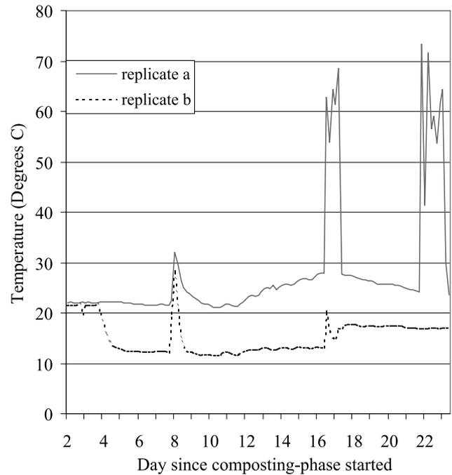
Fig. 2. Temperature profile of the VC-system during the composting-phase.
